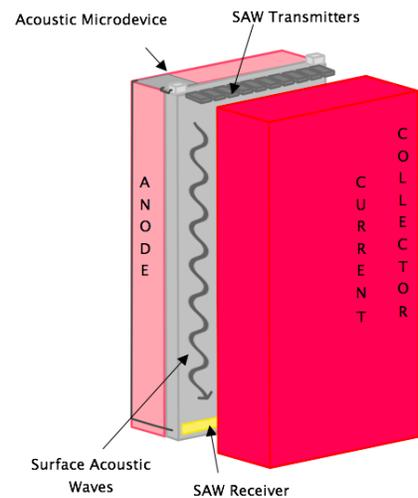
The qSafe system transmits the SAWs along the back of the anode to a corresponding set of receivers. The receivers will detect any changes in the amplitude of the wave and transmit the data to the microprocessor; a drop in amplitude will indicate irregularities on the surface of the anode. If it senses a significant change, the microprocessor prompts the battery to either increase
