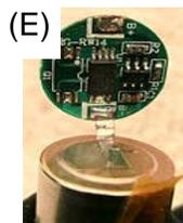
micro device (AMD) consisting of a piezoelectric substance for the SAWs to propagate and an interdigital transducer, which converts electrical signals into acoustic waves. The AMD is attached
